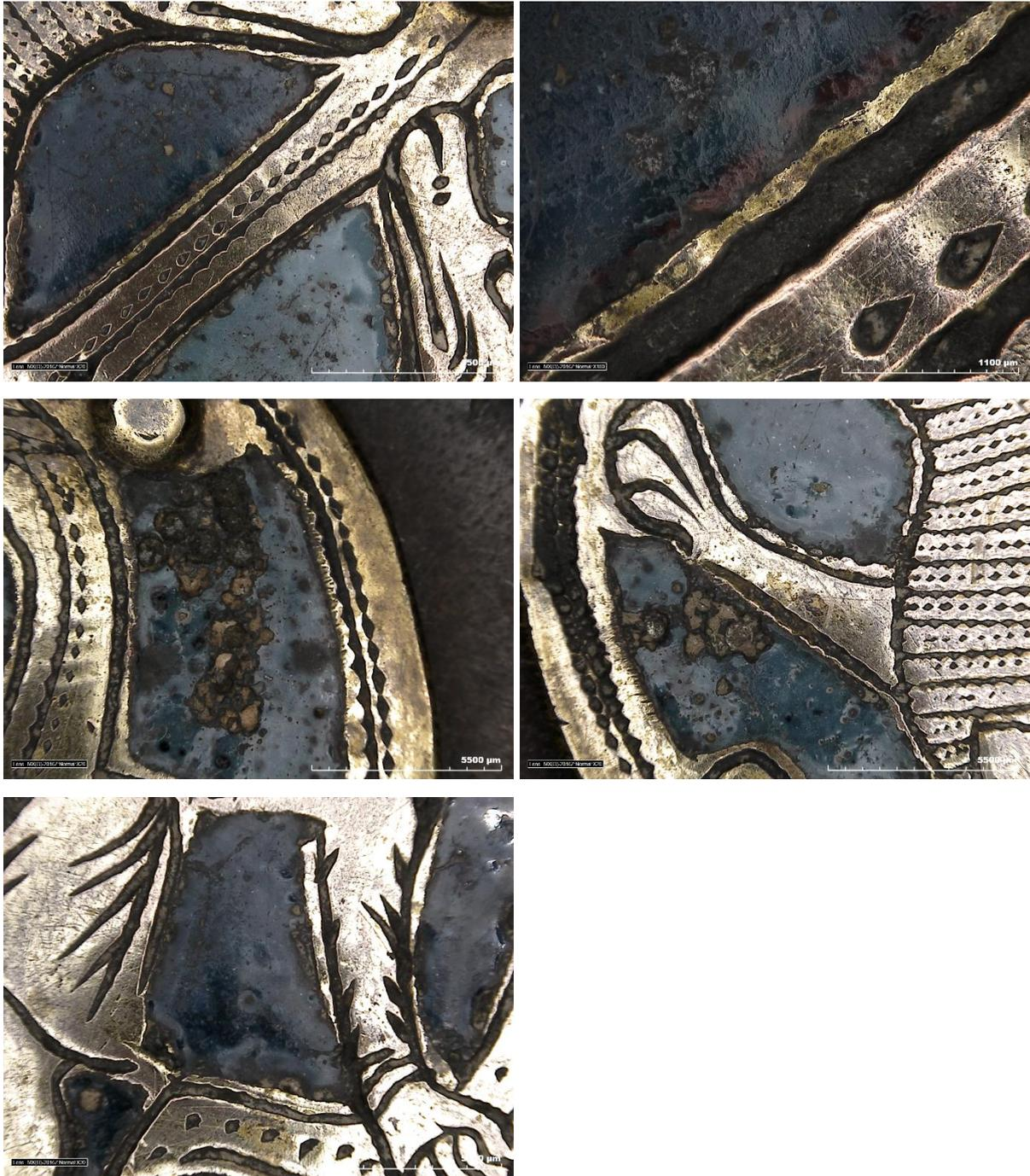
**Figure 20:** Hirox images showing details of medallion 2 (above), medallion 5 (middle, enamel surfaces show pitting corrosion) or medallion 6 (bottom): some parts of the copper have a more yellowish color (presence of gold) compared to other parts.
